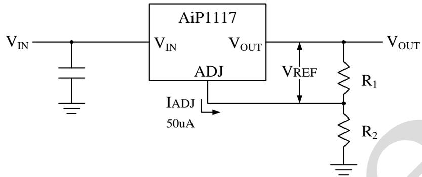
$$V_{OUT} = V_{REF}(1 + R2/R1) + I_{ADJ}R2$$
